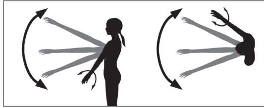
Figure 5 The schematic shows the method of controlling the “third limb” (shown in gray extending out of the participant’s chest). Rotating the right wrist moved the participant’s third limb up and down, whereas rotating the left wrist moved the avatar’s third limb from side to side. Thus, rotating both arms allowed the participant to control the third limb while also hitting targets with the left and right arms.
